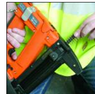
2. Insert collated pin strips. Release magazine tensioner guide.
